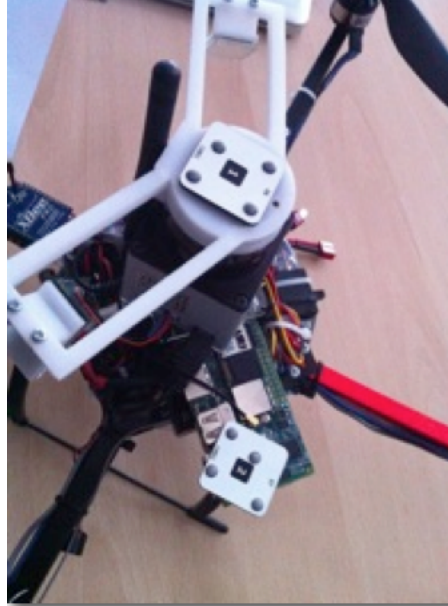
FIG. 29: Two makers are attached in order to calculate position error of VICON system.
